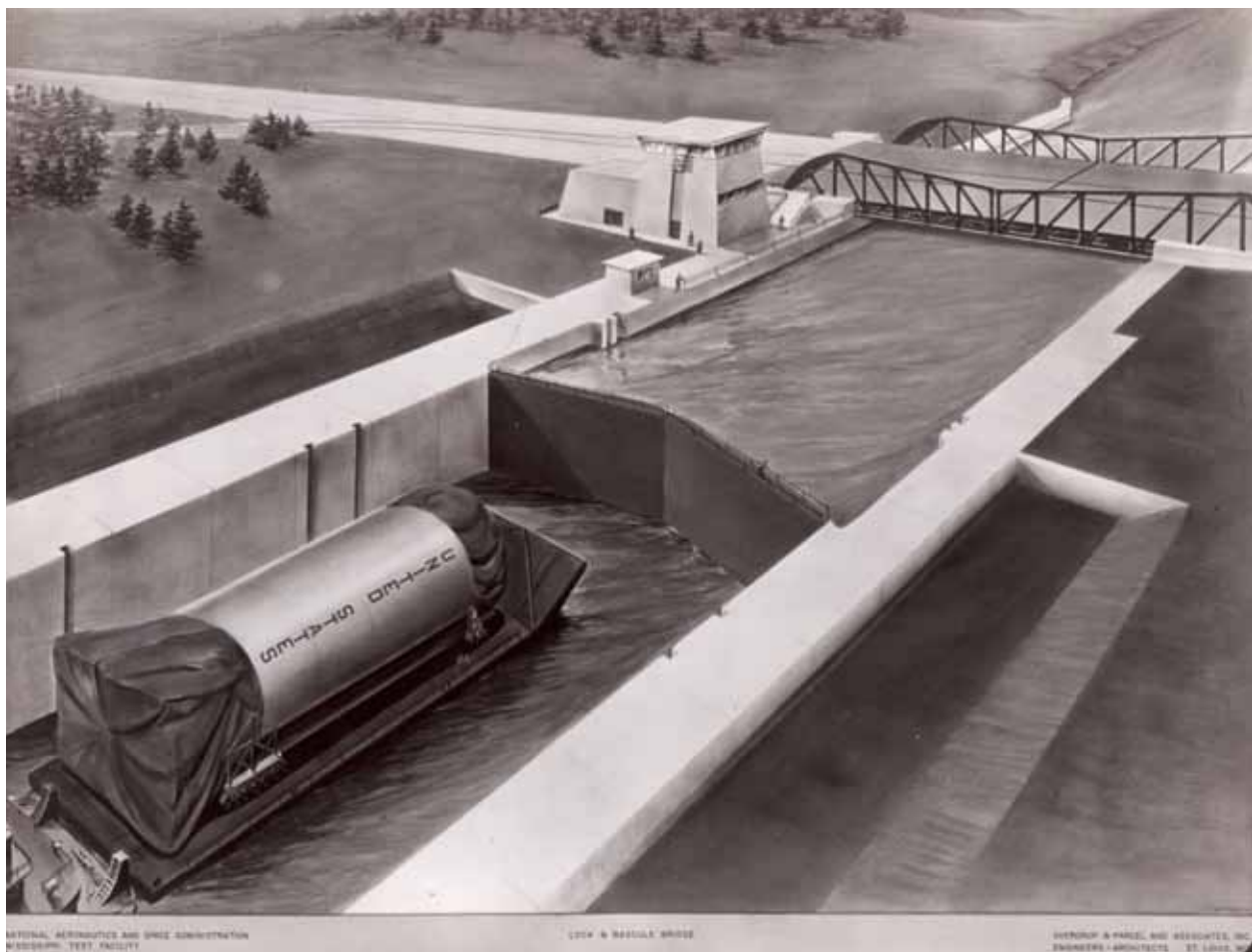
Artist's Concept of Lift Lock and Bascule Bridge at NASA Mississippi Test Facility. Barge transportation potential was important in selecting the site location.
